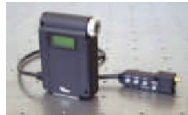
Compact vibration measuring system using diode laser
